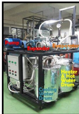
Figure 4. ORC experiment equipment Figure 5. Combination packet of heater & heat exchanger
