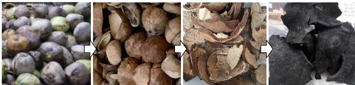
Figure 1. Steps in carbon pyrolysis from coconut shell. Left to right is coconut, coconut shells, chopped and dried coconut shells, and coconut shells after pyrolysis.
