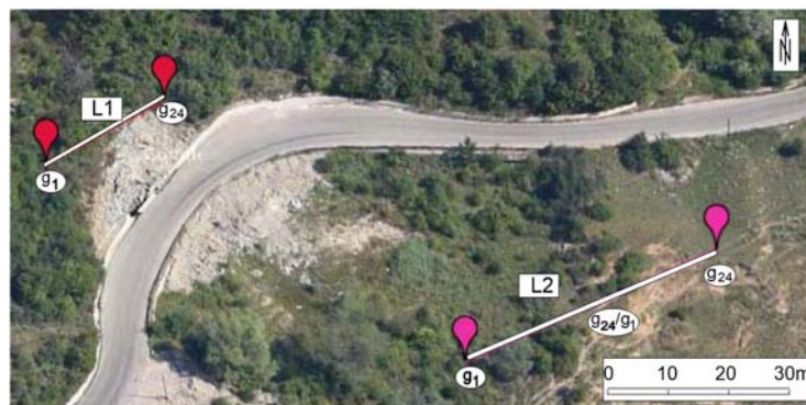
Figure 1. Seismic refraction alignments (L1 and L2) designed over Brebu landslide photo: g1, g24: the end-on receiver places of each spread
