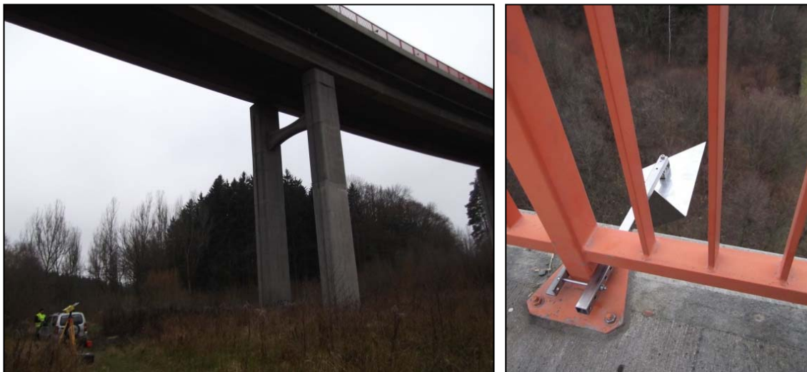
Figure 5 – Measurement situation and corner reflector mounted on the bridge railing
