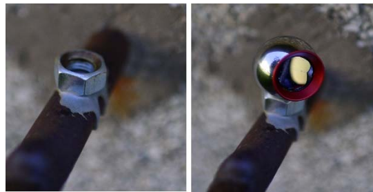
Figure 6. Placement of the 1.5" RRR reflector on a benchmark
