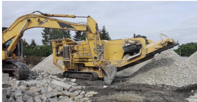
Figure 1. Crushing and screening of concrete waste elements (courtesy Keller Polska)
