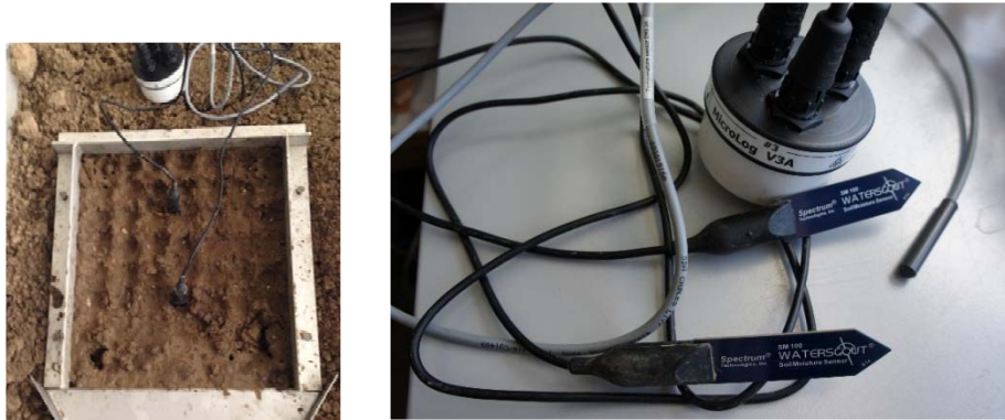
Figure 3. Location of the soil moisture sensors in the test plot
