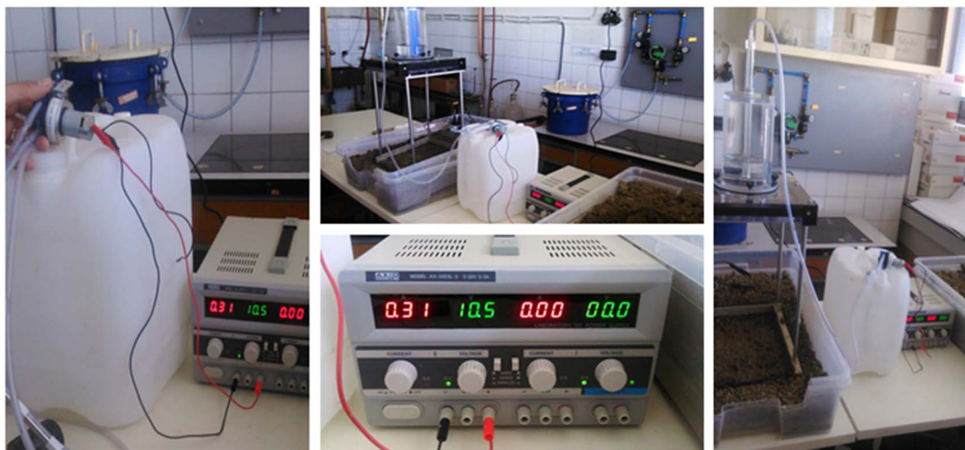
Figure 1. The laboratory equipment used in the experiment. The rainfall simulator was connected to the external source of water, pumped into the reservoir using a peristaltic pump
