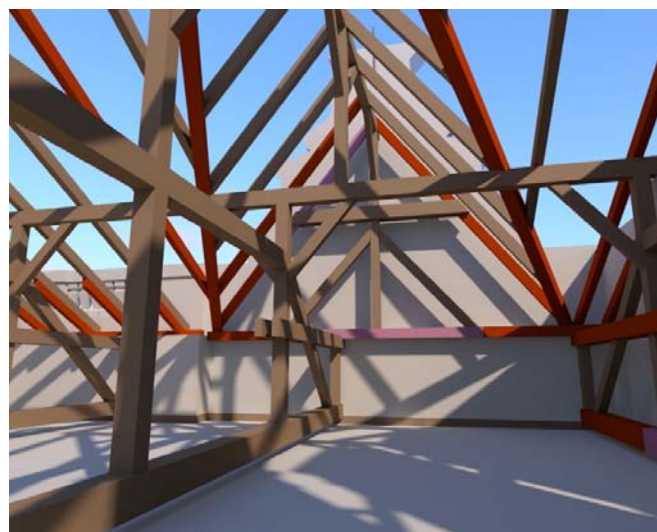
Figure 4. 3D model with highlighted new parts of truss
