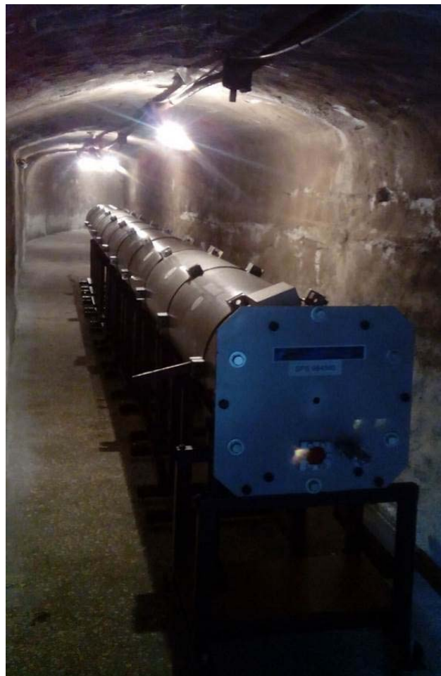
Figure 1. Shock tube in the underground experimental base of the Mining Institute
