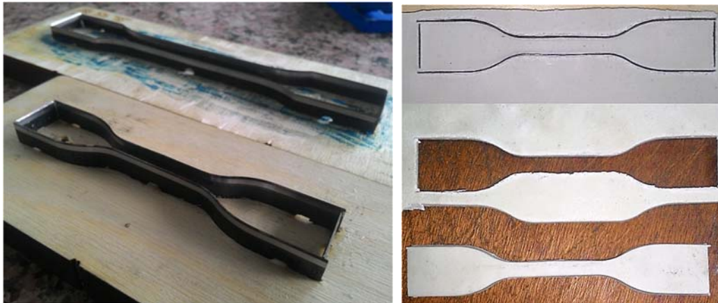
Figure 3. Specimen Preparation by Die cutter
