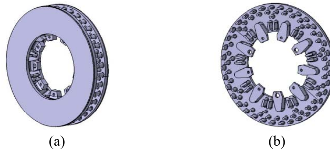
Figure 1. The brake disc model, the left one shows the whole model, and the right one shows the radiating rib structure.
