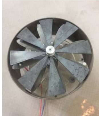
Figure 3. The picture of practical application of the rotary voltmeter
