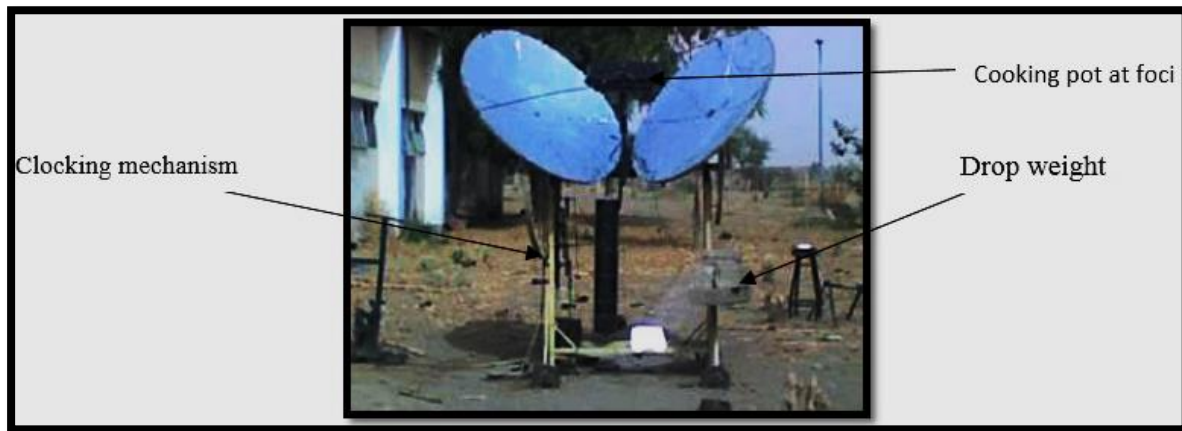
Figure 4. Abdulrahim's bifocal parabolic cooker [36].
