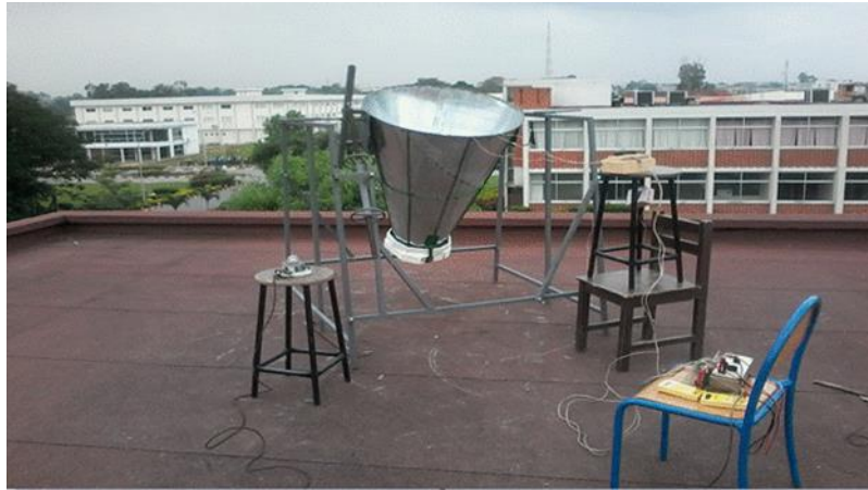
Figure 4. Overall view of the conical solar cooker with accessories on the experimentation site.
