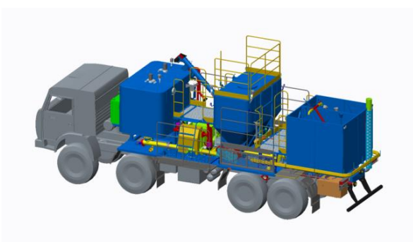
Figure 4. The pumping unit UNB-125x50 SO:
