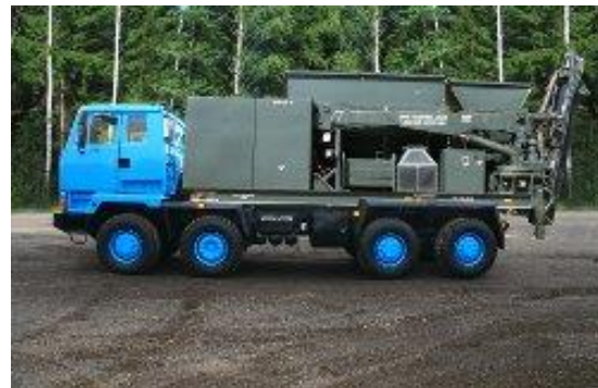
Figure 3. Drilling machine UNB-125x50
