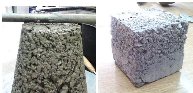
Figure 2. Pervious concrete compaction specifics.
