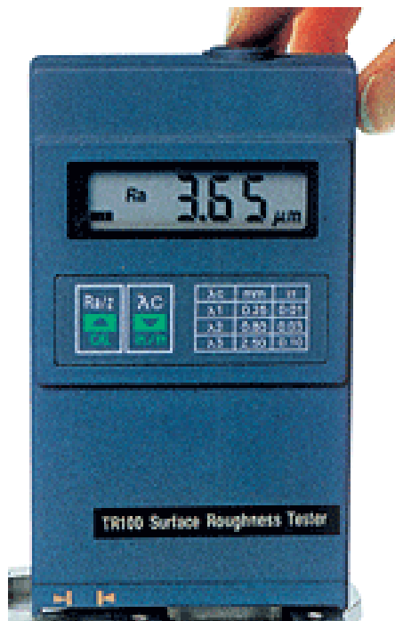
Figure 3. Small-sized TR-100 profilograph. After cutting and turning pump shaft journals, roughness was - Ra 3.2.
