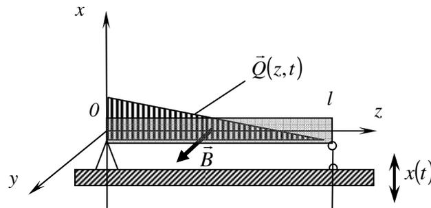
**Figure 1.** Scheme of vibrational system.
