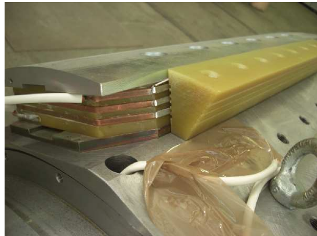
Figure 2. Rotor assembly.
