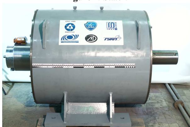
Figure 9. General view of HTS-2G 1 MVA generator.
