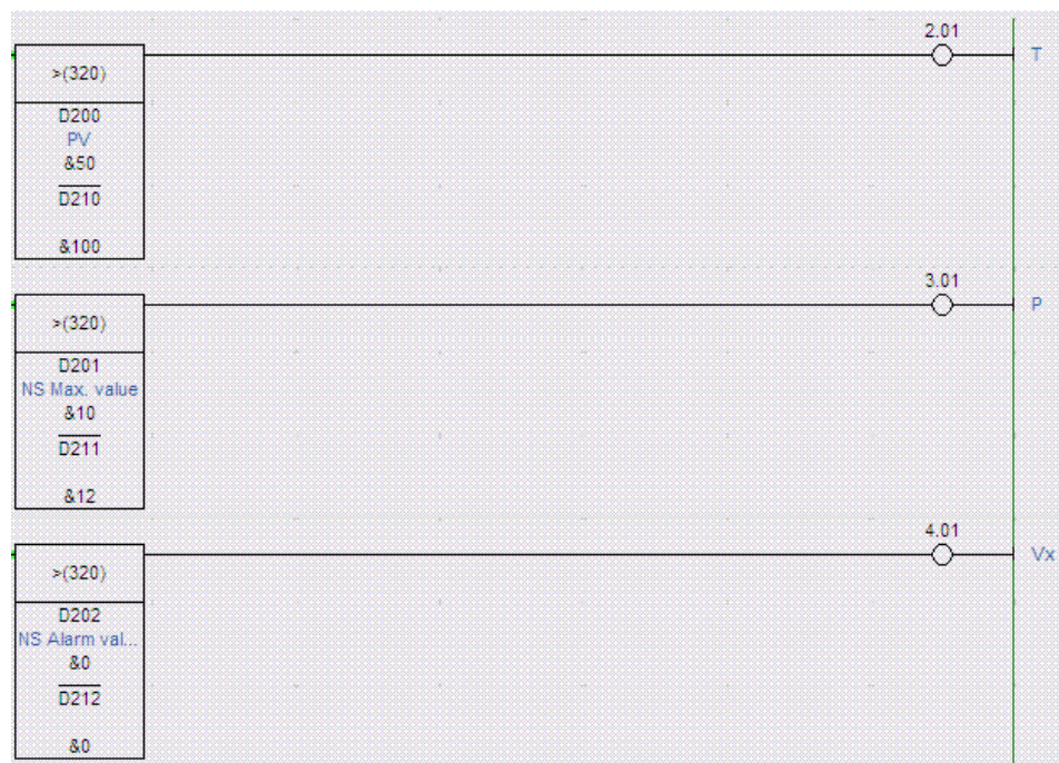
Figure 2. The fragment of the block of conditions for setting permissible parameter values
