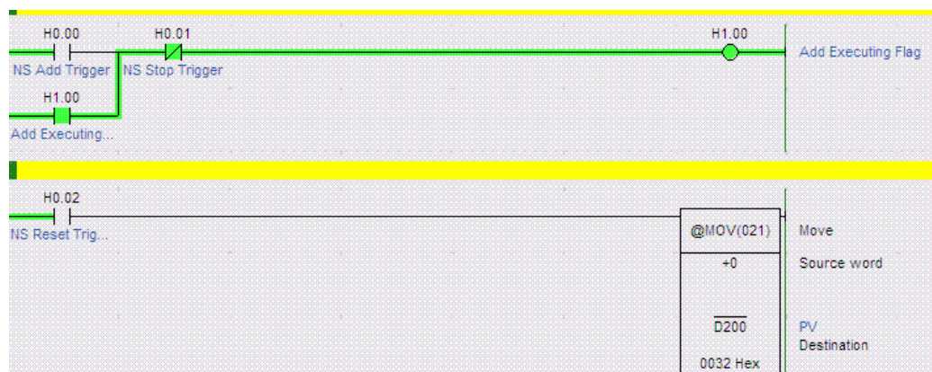
Figure1. The relay-contact diagram for monitoring and controlling the electric drive of the drill. Boom Drive Simulation
