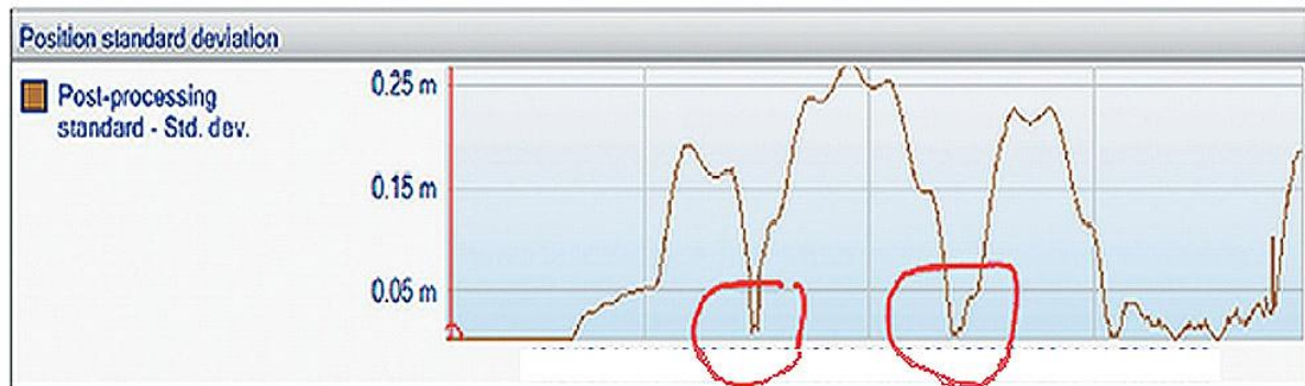
Figure 4: Root-mean-square error of the INS trajectory after adjustment.
