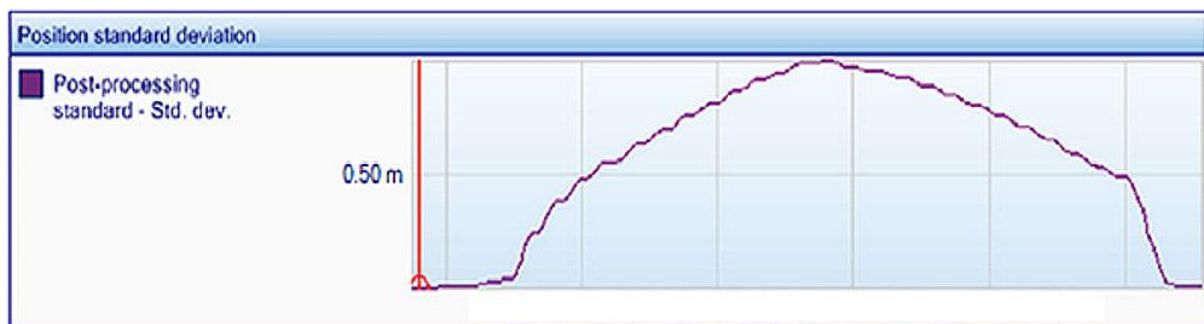
Figure 3: Root-mean-square error of trajectory after processing in forward and reverse directions.
