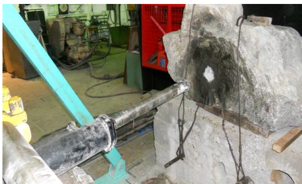
Figure 7. Trial drilling in granite with PNB76U air hammer drill and NKR100M drill rig.
