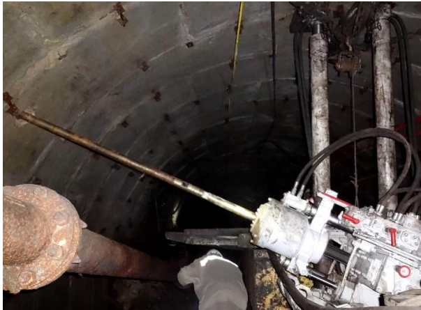
Figure 2. Actual drilling by the drill PNB76 and the drill rig SBR-400 in Berezovskaya Mine, Kemerovo Region.
