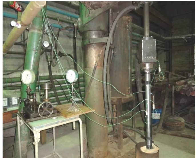
Figure 5. Tests of PNB76U hammer on the vertical test bench GD-251.
