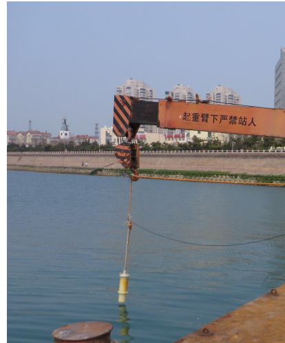
Figure 6. Field measurement of detector ready to be immersed into seawater.
