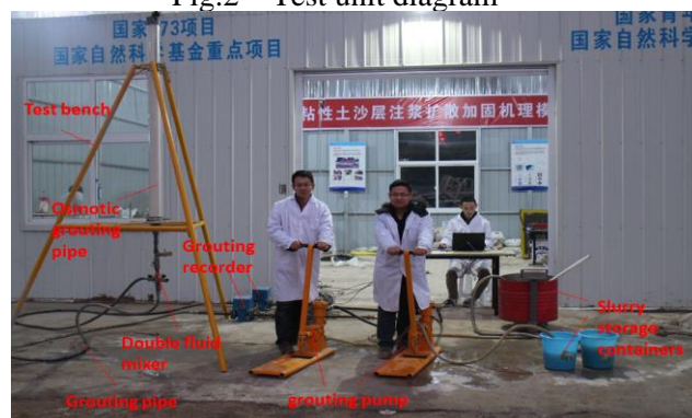
Fig.3 A one-dimensional infiltration grouting simulation test system
