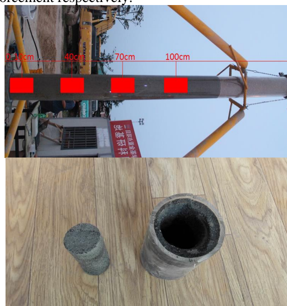
Fig.4 A one-dimensional infiltration grouting simulation test core position
