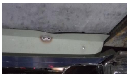
(a) Local buckling of main beam
