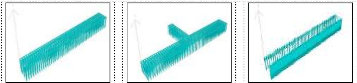
**Figure 6.** Rendered view of piled jetty, piled jetty with approach, diaphragm wall berthing structure.
