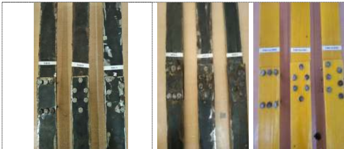
Figure 1. (a) Bolted connection (b) Slot complete penetration welded connection (c) Bolted connection in GFRP.
