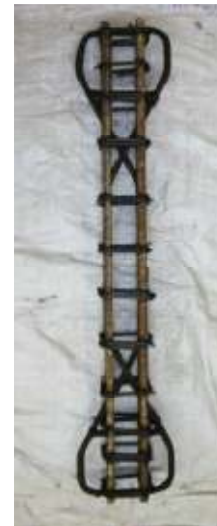
Figure 3. Typical reinforcement arrangement for the column
