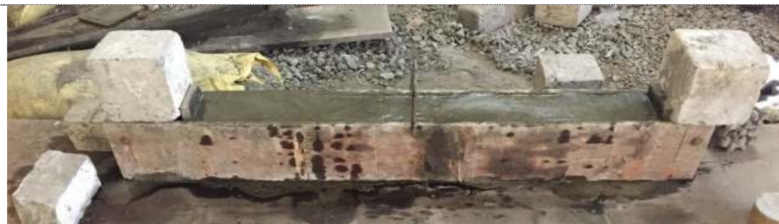
Figure 2. Flexural member concrete placement for 25% OBB
