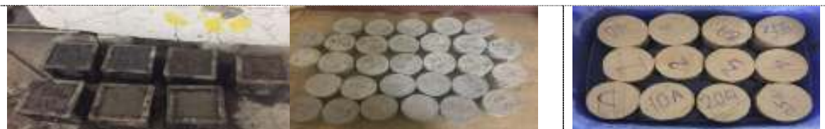
Figure 1. Concrete specimens for compressive strength and durability test
