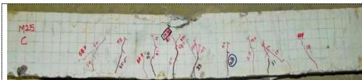
7(a). Crack pattern for M25 Control beam
