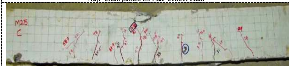
7(b). Crack pattern for M25 optimum mix (FA+SF)-2 beam
