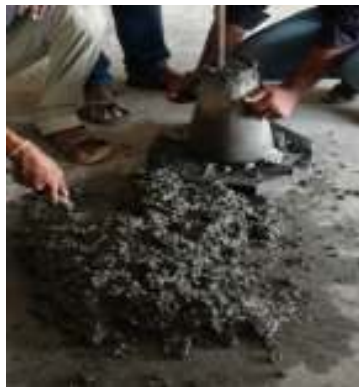
Figure 1. Slump Test
