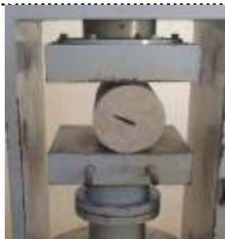
(b) Split Tensile Test
