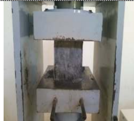
Figure 3. Specimen under compression
