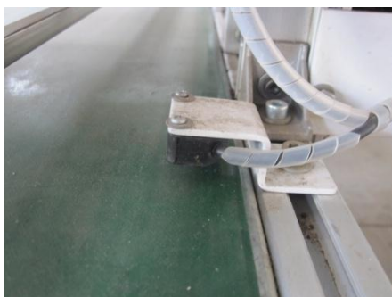
Figure 2. Photo-reflect zone of the conveyor.
