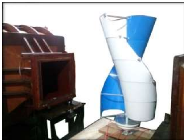
Figure 1. Wind Turbine Testing Using Wind Tunnel.
