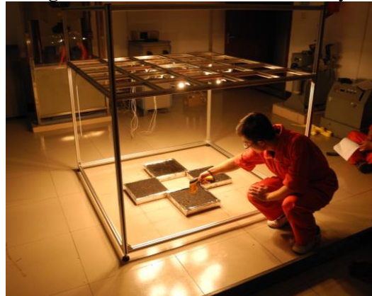
Figure 6: Test of surface temperature and permeability coefficient.
