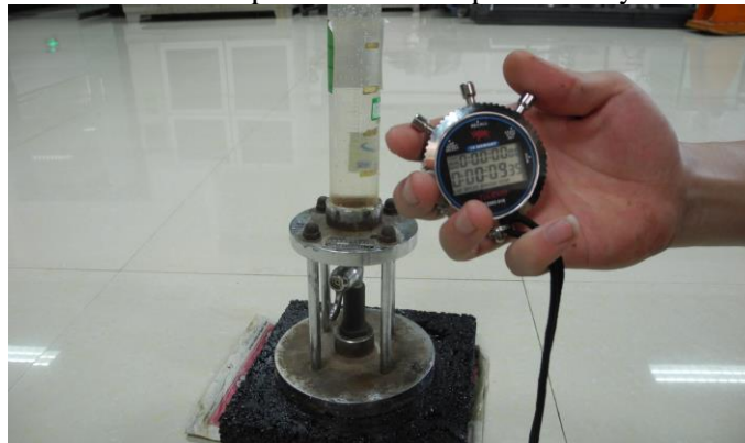
Figure 2: Permeability tests in laboratory.
