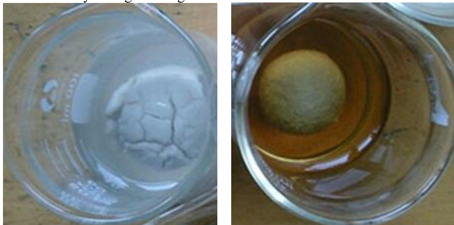
Fig.3 The status of mud balls immersed in water (left) and 5% CG (right) solution for 48 h
