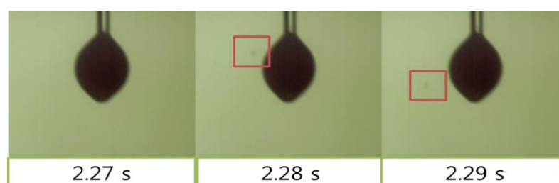
Figure 4. Micro explosion phenomenon of a droplet at 800°C
