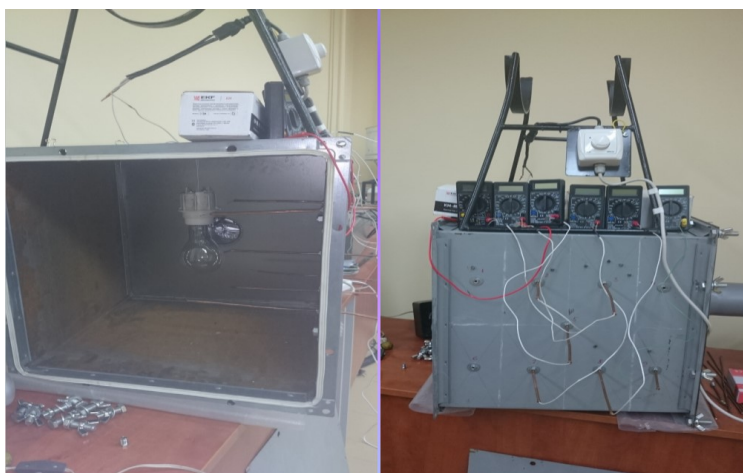
Figure 1 – The experimental setup for the study of different types of heat transfer
