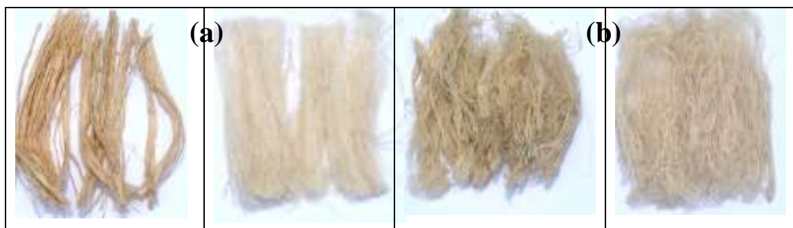
Figure 2. The Ramie Fiber : (a) middle part (before and after biodegumming) (b) end of the fiber (before and after biodegumming)
