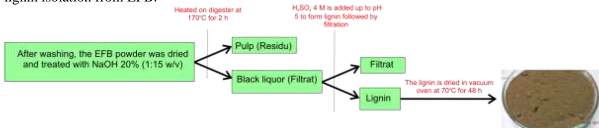
Figure 3. Lignin isolation technique from Empty Fruit Bunch (EFB) of Oil Palm
