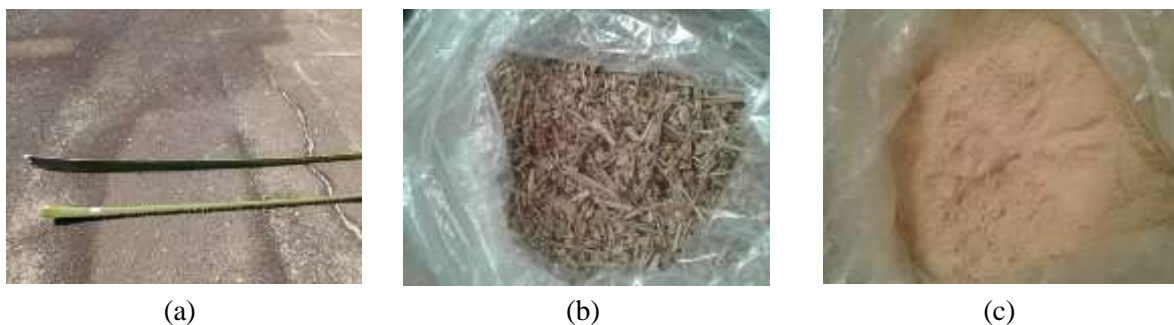
Figure 1. (a) Fresh palm frond (b) Palm frond after chopping (c) Palm frond after powdering
