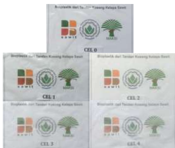
Figure 8. Transparency of the EFB bioplastic with different cellulose content: 0%, 12.5%, 25%, 37.5%, 50% and 75%.
