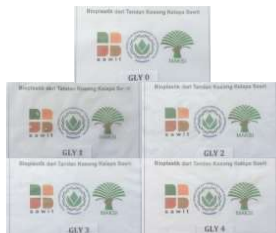
Figure 9. Transparency of the EFB bioplastic with different glycerol content: 0%, 12.5%, 25%, 37.5% and 50%.
