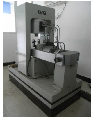
Figure 1. RMT-150C rock mechanics test system
