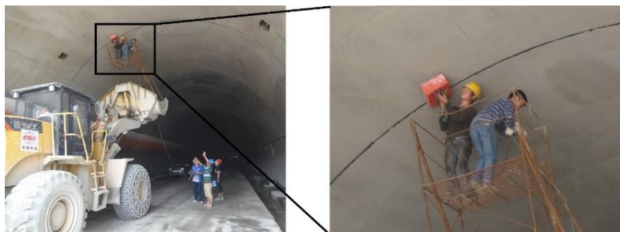
Figure 6. Data collection during the field quality inspection of Yushan tunnel lining
