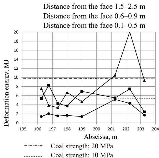
**Figure 5.** Energy deformation of coal under rock pressure.
