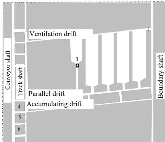
**Figure 1.** Automated coal mining with short rooms.
