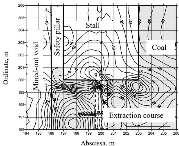
**Figure 2.** Isolines of vertical stresses (MPa) in the immediate roof rocks at the juncture of the shortwall and stall.
