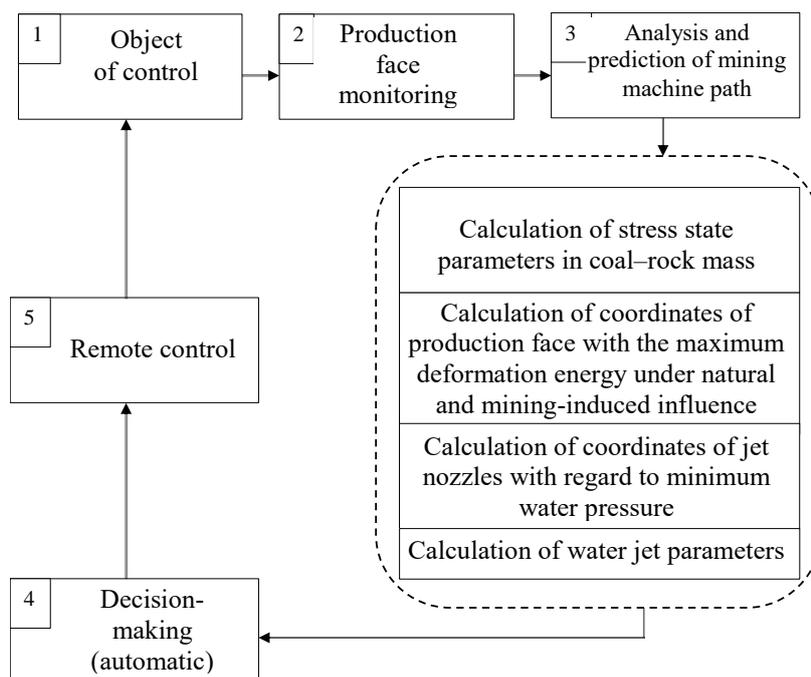
**Figure 4.** Flow chart of remote control of coal shortwalling.
