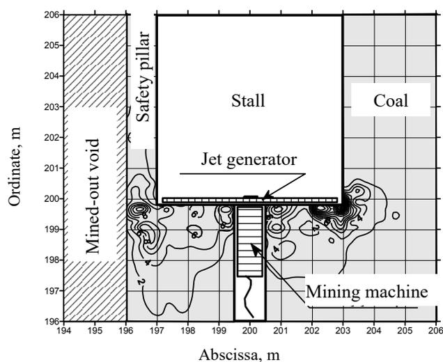
**Figure 3.** Isolines of the deformation energy (MJ) in coal bed at the juncture of the shortwall and stall.
