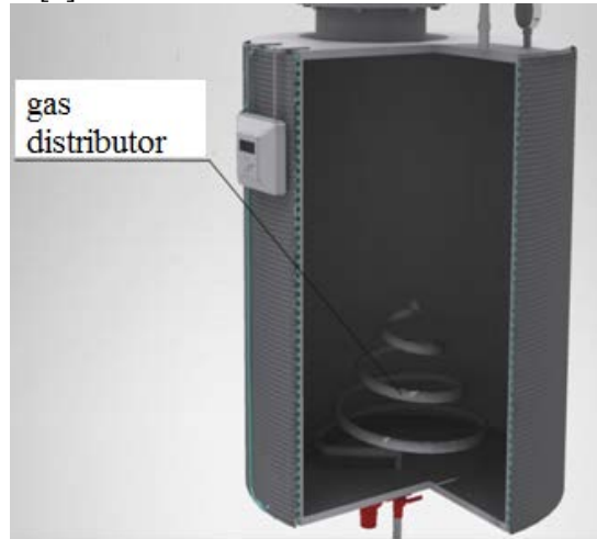
Figure 1. The bioreactor with system of hashing of bubbling type.
