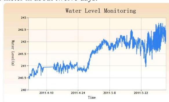
Figure 4. CAISM real time water level monitoring data
