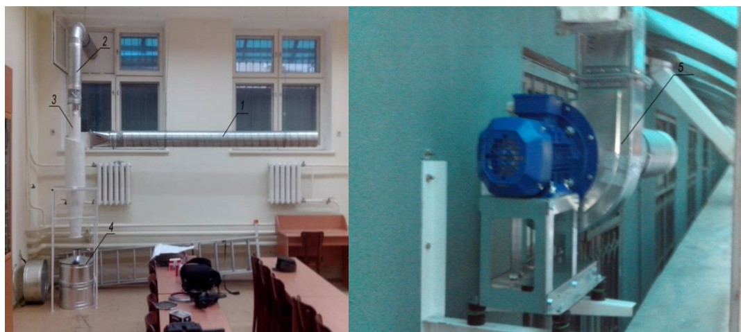
Figure 1 – Experimental plant «Cyclone»: 1 – inlet pipe, 2 – outlet pipe, 3 – Cyclone CN-15-300 (through quick release clamps can be easily replaced to COK), 4 – hopper, 5 – round blower
