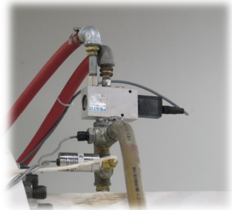
Figure 6: Pressure control apparatus on the upstream tank
