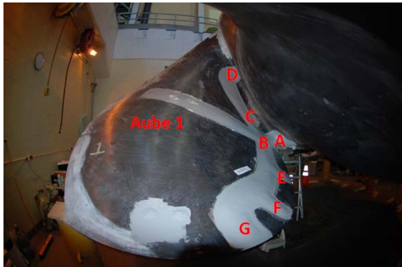
Figure 1. Instrumented runner blade with protective coating and gauge sites
