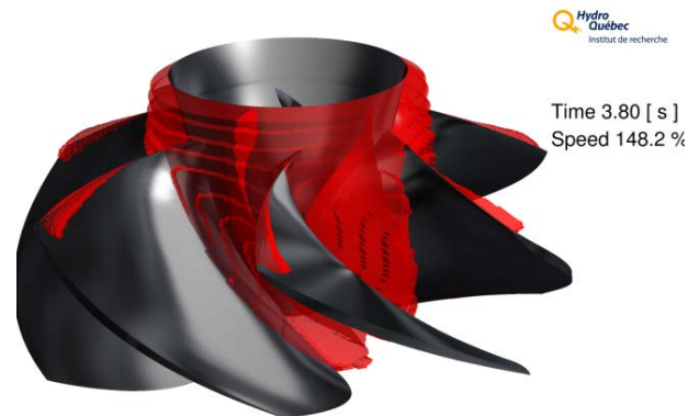
Figure 9. Iso-volumes of negative absolute pressure at maximum speed
